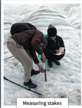
Drilling using Heucke Drilling machine
